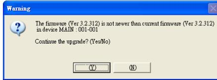
If you didn't enable *Check Firmware Version*, the utility installs the upgrade files without checking whether they are a higher level, or not.
