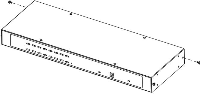
2. Use the M3 x 8 Phillips head hex screws supplied with the rack mount kit to screw the rack mounting brackets into the sides at the rear of the unit.
