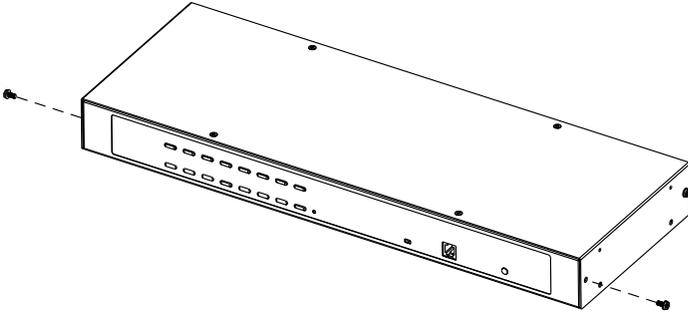
2. Use the M3 x 8 Phillips hex head screws supplied with the rack mount kit to screw the rack mounting brackets onto the side panels near the front of the unit.
