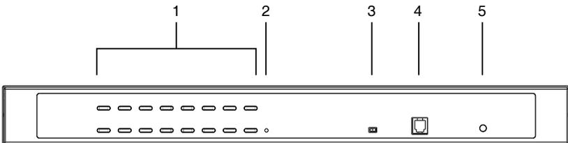
**Note:** The CS1316 is pictured above. The CS1308 / CS1308D front panel is the same as the CS1316, except that it has 8 KVM port LEDs instead of 16.
