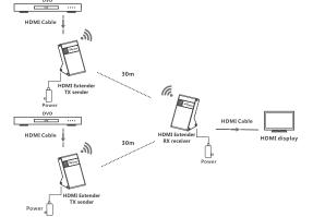
Note: When the transmitter and the receiver are placed face to face of each other, the transmission distance is up to 30 meters; when the transmitter and the receiver are placed freely, transmission distance is up to 8meters.
