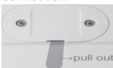
First, remove the plastic ring from the battery space at the rear of the metre, as shown in the picture. The installed batteries 2x 1.5V (LR44/AG13) are used to power the metre memory.
