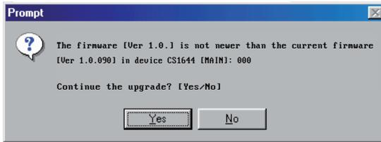
If you enabled *Check Firmware Version*, the Utility compares the device's firmware level with that of the upgrade files. If it finds that the device's version is higher than the upgrade version, it brings up a dialog box informing you of the situation and gives you the option to Continue or Cancel.
